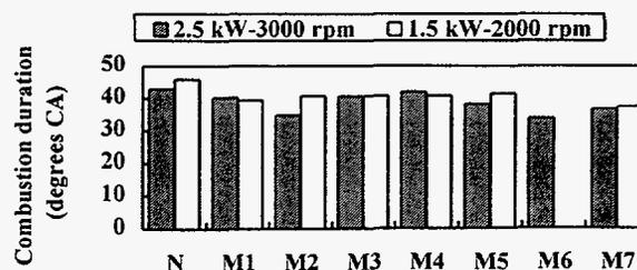
Fig. 9 Comparison of combustion duration for different modifications
