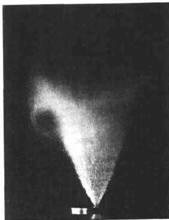
Plate 7.4 A spray pattern from an optimized liquid fuel injection system (courtesy of Mercury Marine).
