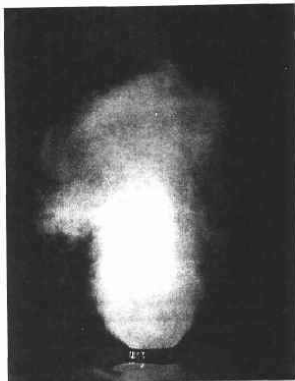
Plate 7.5 A spray pattern from an optimized air-assisted fuel injection system (courtesy of Mercury Marine).
