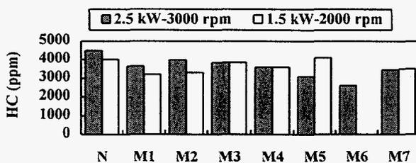
Fig. 6 Comparison of hydrocarbon emissions with different modifications
