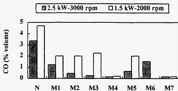
Fig. 5 Comparison of carbon monoxide emissions for different modifications
